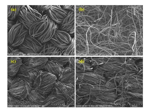
Figure 5. SEM images showing the weave pattern of: (a) polyester (b) fleece (c) cotton and
