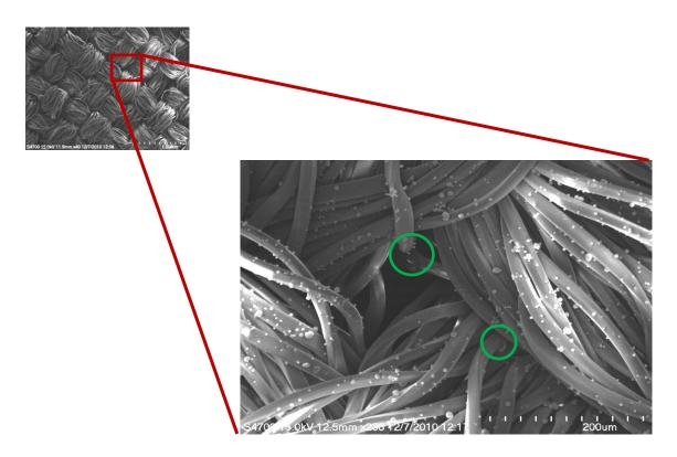
*Figure 6. SEM image of particles deposited deep into the weave (circled areas) of contaminated polyester*
