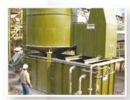
**Burnley Baffles** are our internationally patented dust suppression device designed to reduce the escape of dust from dump hoppers and chutes handling dry granular bulk raw materials such as grains and ores. A **Burnley Baffle** installation consists of a set of modules that fill the open inlet face of a hopper.
